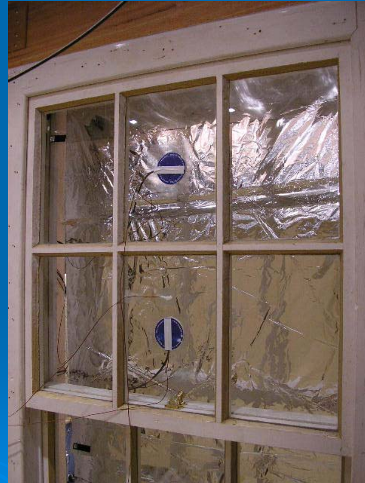
Blind with low-e foil applied
